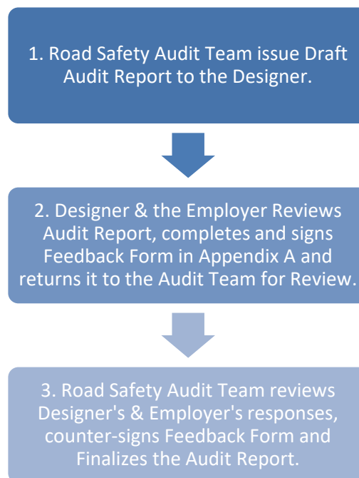
Figure 4.1 – Road Safety Audit Sign-Off and Completion Process
