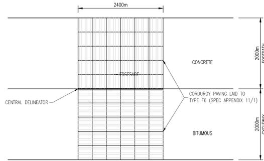
**CYCLEWAY & FOOTPATH TACTILE PAVING PLAN**
