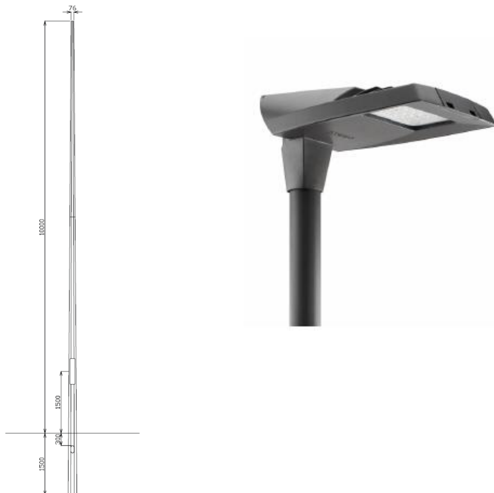
Figure 2.1 Typical Public Column and LED Head
