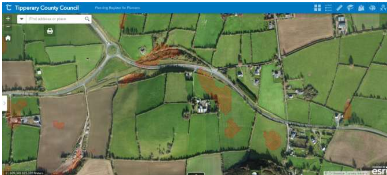
Figure 4 Areas identified at risk of pluvial flooding (hatched in red)
