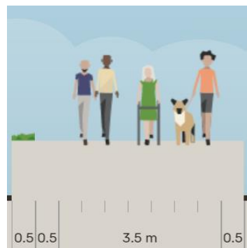
Figure 3-5: Davnets Row shared path cross section
